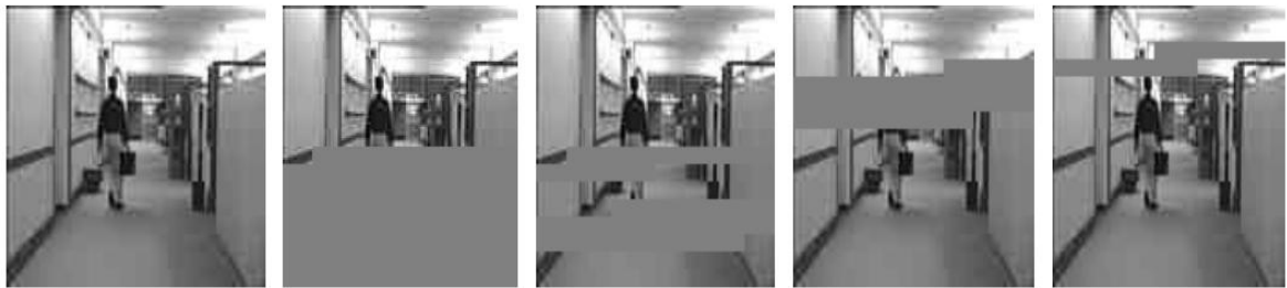
(a) Transmitted frame (b) 1-path, g=0 (c) 2-path, g=0 (d) 1-path, g=15 (e) 2-path, g=15 PSNR=29.530 PSNR=20.1803 PSNR=22.1850 PSNR=19.819 PSNR=24.319 SSIM=0.907 SSIM=0.747 SSIM=0.802 SSIM=0.767 SSIM=0.850
